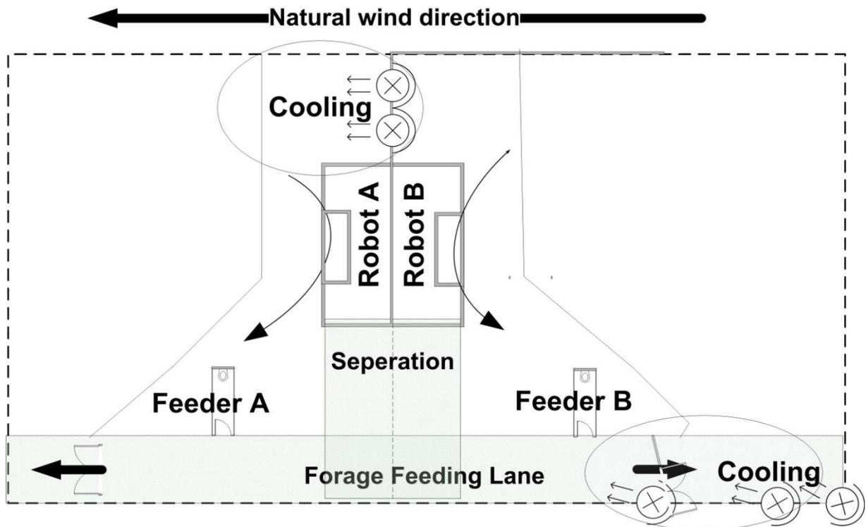
Figure 1. Experiment design and farm layout. Two cow groups milked by two robots located in the centre of the cowshed. The arrows pointing are the cow gait direction. The cows are separated, cows from group A can be milked only in robot A and vice versa – cows from group B can be milked only by robot B.
